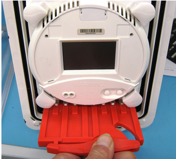
Installing the Paddle Board
