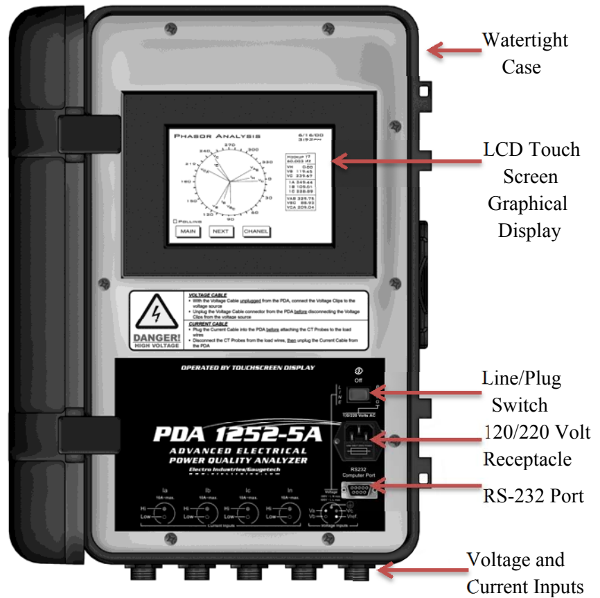
Figure 2.2: The PDA 1252 Opened
