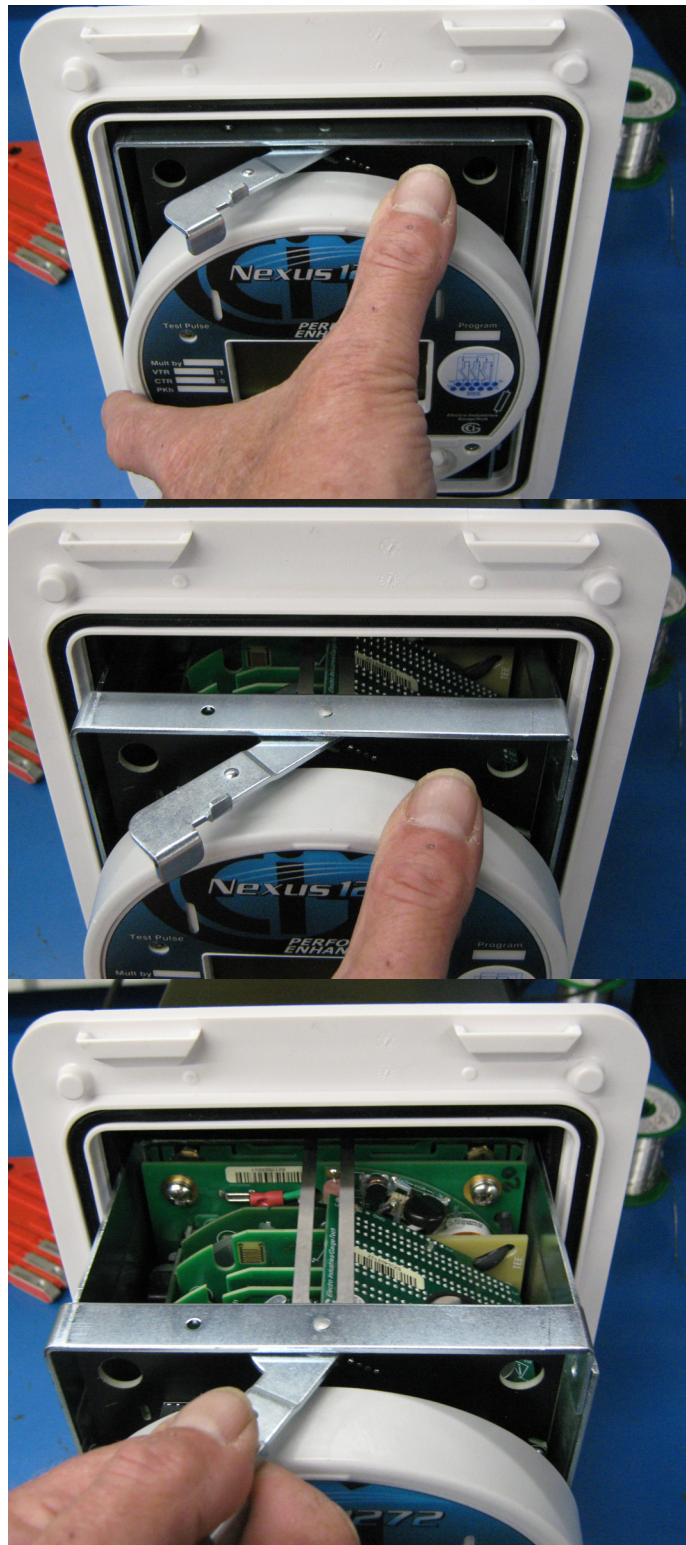
Figure 6.14: Removing the Meter Cradle
