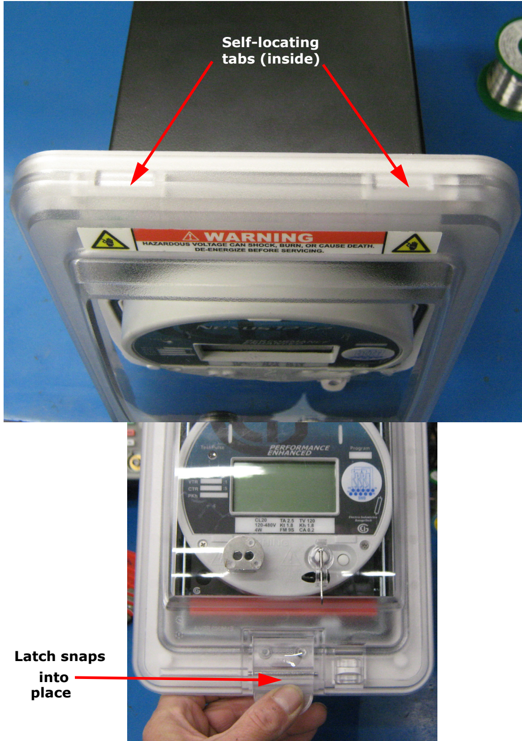
Figure 6.18: Reinstalling the Bezel
