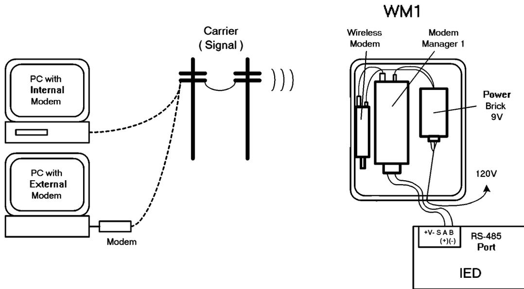
Figure 2.1: WM1 Wireless Modem Kit Installation
