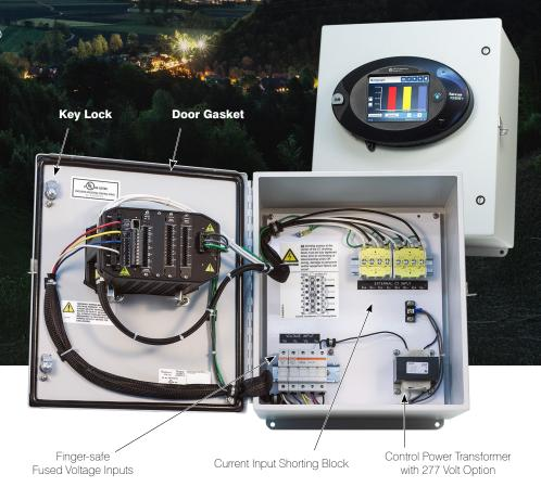
EIG's Nexus<sup>®</sup> 1500+ meter in enclosure lets you expand your switchgear capability without expensive and time-consuming redesign. Simply mount and wire the enclosure next to your switchgear and you are ready to go, with no downtime at all! This is a perfect solution for a retrofit when there is no metering compartment available.
